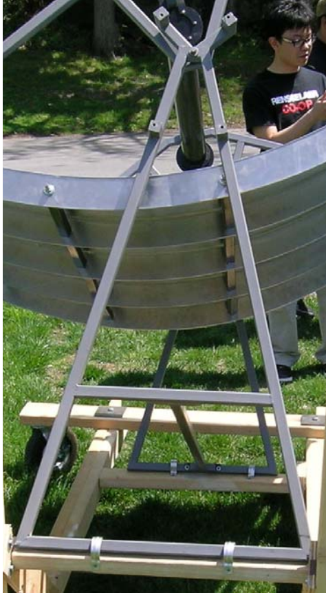
Figure 30: Current frame design (high side)
