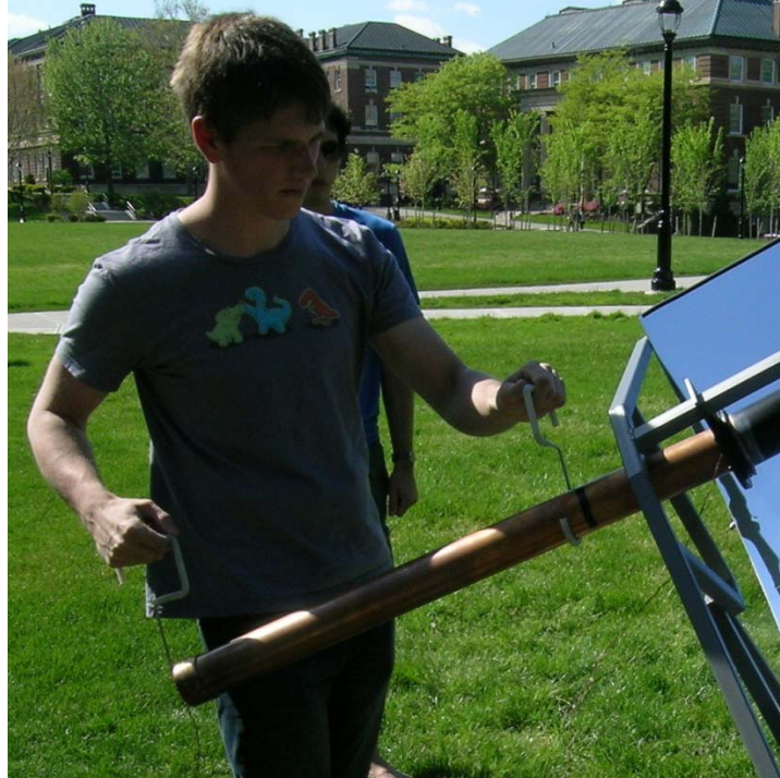
Figure 16: Henry Wetterson shown using the 'hay hooks' to remove the reactor insert
